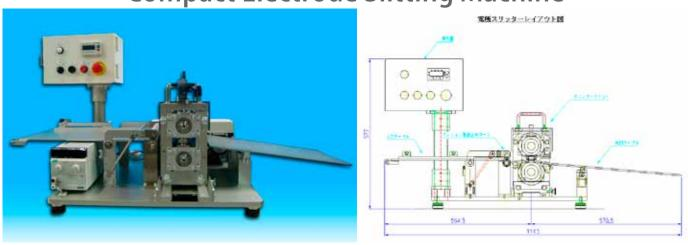
This equipment is used for slitting a pre-cut electrode sheet of LIB, EDLC, LIC and etc. Setting the pre-cut electrode sheet by hand and pressing start button of the equipment, the sheet is automatically fed into slitting unit and completely cut to two or three stripes.
