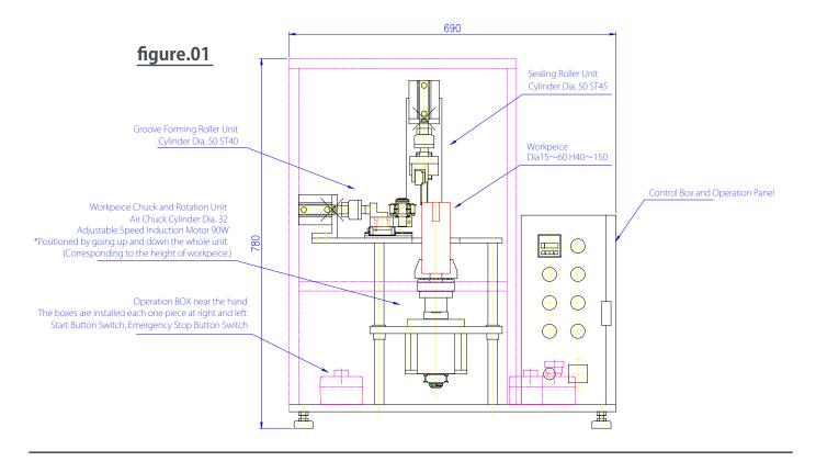
This machine is to seal the Cylindrical Cells.
